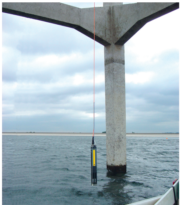
A YSI multiparameter water quality sonde is fixed to, and lowered from, a tower in the Queen Mother Reservoir. It will profile the entire water column of the reservoir.
